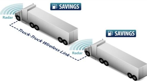
The two trucks are able to get as close as 20 feet from each other while platooning in order to take advantage of fuel-saving aerodynamics. Peloton reports fuel savings of 10% for the second truck and 4.5% for the lead truck in a platoon. The trucks are able to get this close thanks to Peloton's active safety system which wirelessly links the trucks. The wireless link controls the truck's acceleration and braking, while radar detects potential dangers up ahead.
